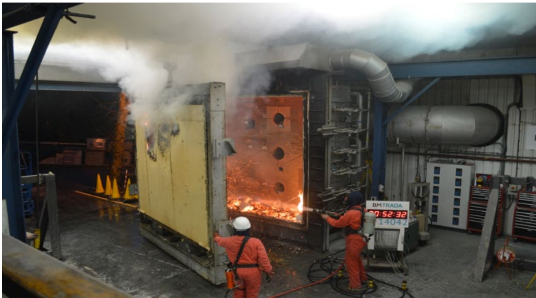
Fig 3 A fire resistance test performed on a loadbearing timber framed straw insulated wall system
