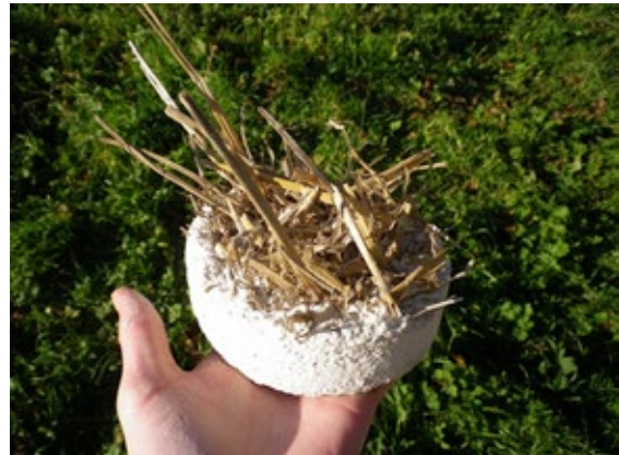
Fig 5 Render core removed from three year old straw bale panel
